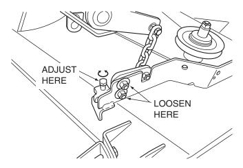
Figure 6-5. Cutter Deck Level Adjustment
